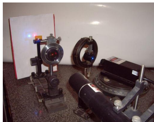
Figure 2. Experimental setup for photoinduced birefringence measurement.
